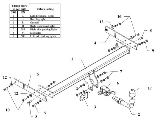
This towing hitch is designed to assembly in following car: **VOLKSWAGEN TIGUAN**, produced since 2007, catalogue number **K51A** and is prepared to tow trailers max total weight **2000 kg** and max vertical mass **100 kg**.
