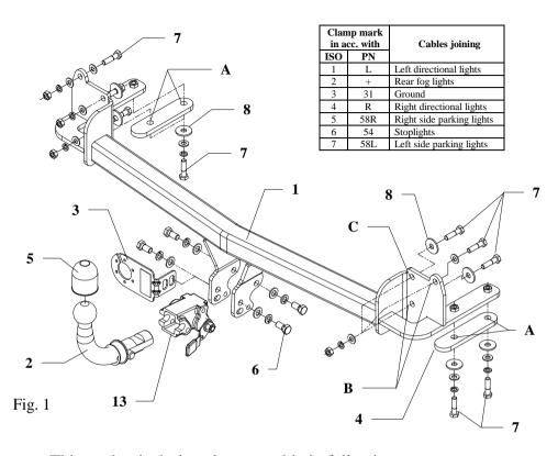
This towbar is designed to assembly in following car: MAZDA PREMACY produced since 10.1999 till 2005, catalogue no. M43A and is prepared to tow trailers max total weight 1600 kg and max vertical load 50 kg.
