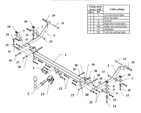
This towing hitch is designed to assembly in following cars: **FIAT DUCATO L4, PEUGEOT BOXER L4, CITROEN JUMPER L4, metal built-up,** produced since 2006, catalogue no. **R42A** and is prepared to tow trailers max total weight up to **3100 kg** and max vertical load **124 kg**.
