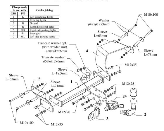
This towing hitch is designed to assembly in following cars: **NISSAN MICRA, 3/5 doors (K11),** produced since 08.1992 till 2002, catalogue no. **V50A** and is prepared to tow trailers max total weight **1150 kg** and max vertical load **50 kg**.
