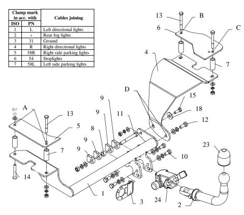
This towbar is designed to assembly in following cars: **SUZUKI SWIFT** produced since 2005, catalogue no. **W21A** and is prepared to tow trailers max total weight **1100kg** and max vertical load **50kg**.
