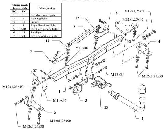
This towing hitch is designed to assembly in following cars: SUZUKI GRAND VITARA, 3 doors, produced since 2005, catalogue number W24A and is prepared to tow trailers max total weight 1600 kg and max vertical load 85 kg.
