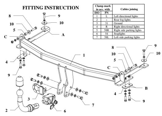
This towbar is designed to assembly in following cars: HONDA JAZZ, produced since 2002 till 2008, catalogue no. Y27A and is prepared to tow trailers max total weight up to 1000 kg and max vertical mass 70 kg.
