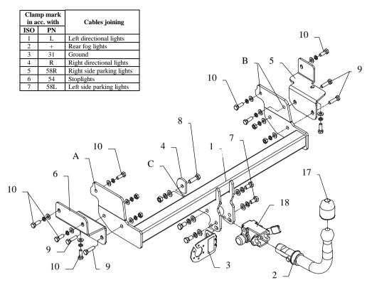
This towbar is designed to assembly in following cars: MITSUBISHI LANCER ESTATE produced since 06.2003 till 2008, catalogue no. Z30A and is prepared to tow trailers max total weight 1200 kg and max vertical load 60 kg.
