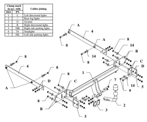
This towing hitch is designed to assembly in following cars: MERCEDES C-CLASS SEDAN (W204) produced since 03.2007 and ESTATE (S204) produced since 11.2007, catalogue number D38 and is prepared to tow trailers max total weight 1800 kg and max vertical mass 100 kg.
