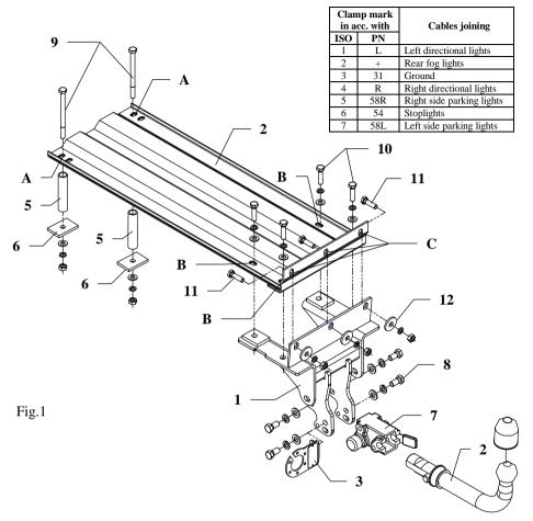
This towbar is designed to assembly in following car: **OPEL OMEGA "B" 4 doors,** produced since 04.1994, catalogue no. **E16A** and is prepared to tow trailers max total weight **2100 kg** and max vertical load **75 kg**.
