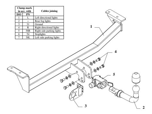
This towbar is designed to assembly in following cars: **TOYOTA YARIS VERSO**, produced since 2000 till 2006, catalogue no. **O16A** and is prepared to tow trailers max total weight **1000 kg** and max vertical load **50 kg**.
